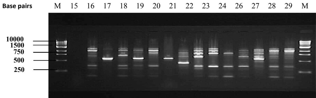
**Figure 1.** (b) Agarose (1.2%) gel electrophoresis of RAPD-PCR products for primer Gold Oligo OPAR3 of *V. parahaemolyticus* isolates. Lanes : M, 1kb ladder ; 15, VP15; 16, VP16; 17, VP17; 18, VP18; 19, VP19; 20, VP20; 21, VP21; 22, VP22; 23, VP23; 24, VP24; 25, VP25; 26, VP26; 27, VP27; 28, VP28; 29, VP29
