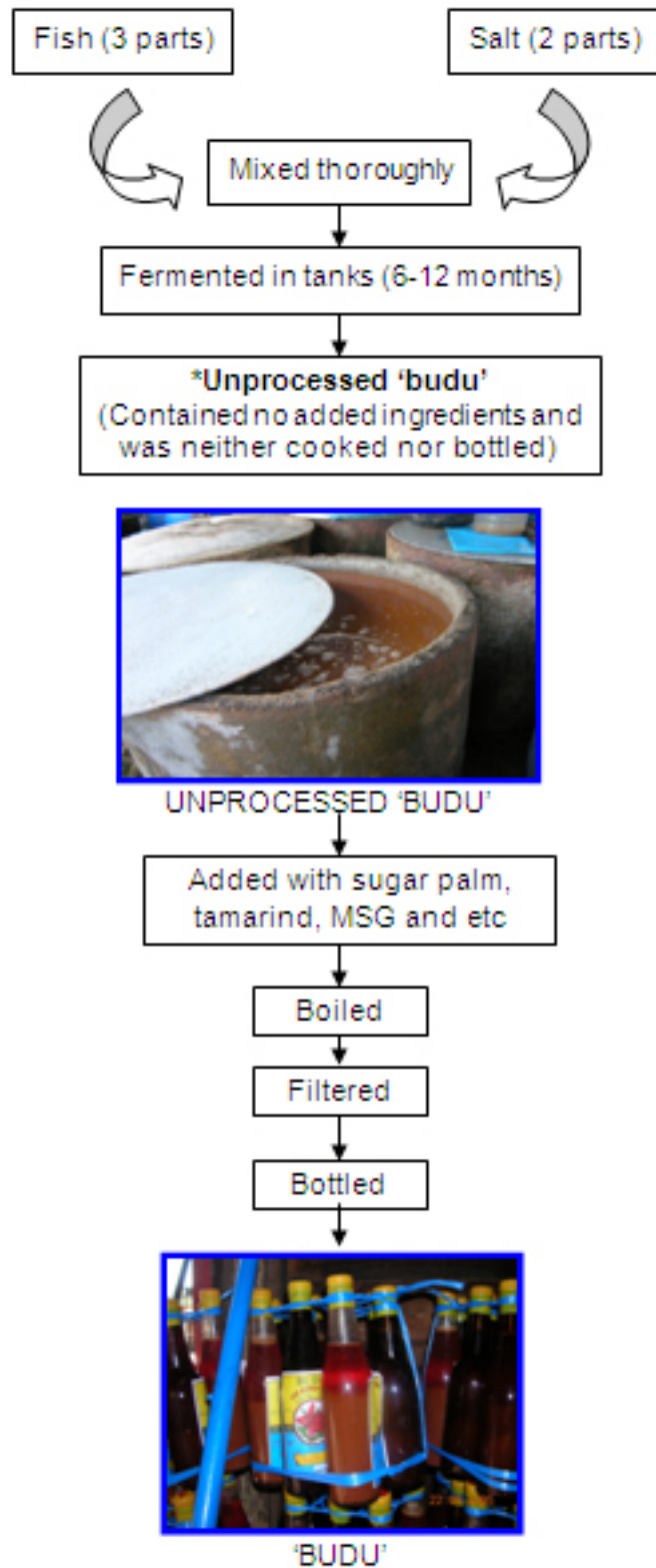
Figure 1. Flow chart for production of Malaysian 'budu'. * indicates sample used in this study
