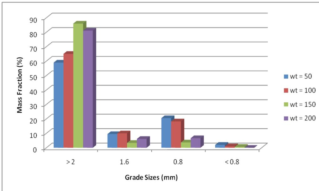
**Figure 3.** Effect of feed weight on particle size distribution of the tapioca globules
