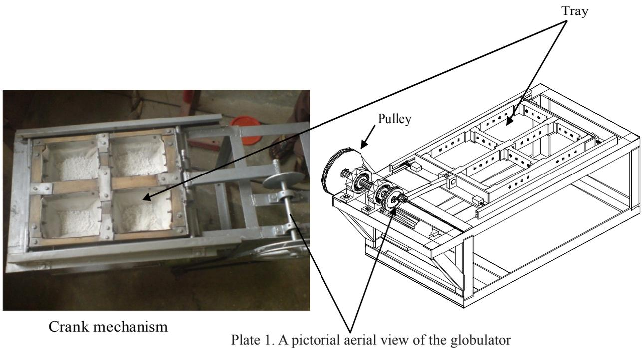
Figure 2. Isometric view of the globulator.
