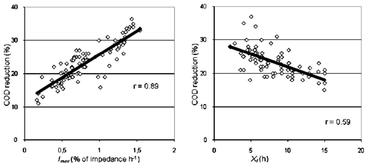
**Figure 4.** Correlations between the values of COD reduction obtained in the result of shaken cultures and parameters of the dynamics of electrical impedance changes ( $I_{max}$  and  $X_l$ ) recorded during wastewater biodegradation by the tested microorganisms
