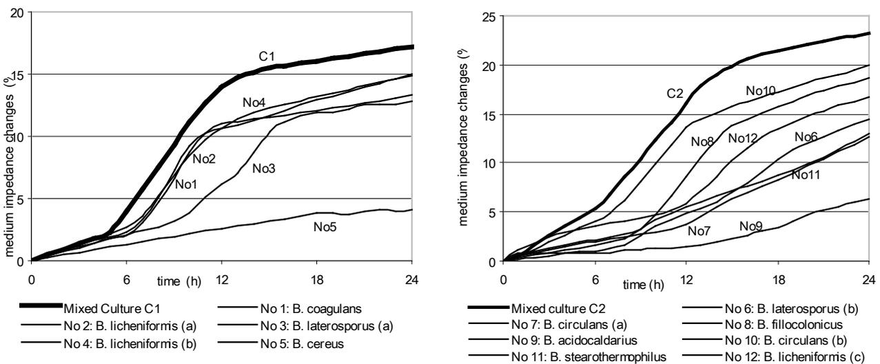
**Figure 3.** The course of electrical impedance changes during starch wastewater biodegradation by using of *Mixed Cultures C1* and *C2* and single isolates coming from them.
