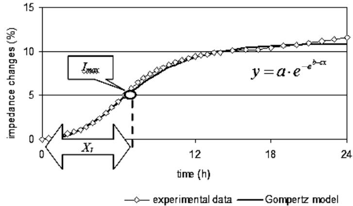
**Figure 1.** Mathematical description of the electrical impedance changes data obtained during bacterial wastewater biodegradation
