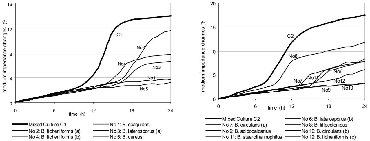
**Figure 2.** The course of electrical impedance changes during hot wastewater biodegradation by using of *Mixed Cultures C1* and *C2* and single isolates coming from them.
