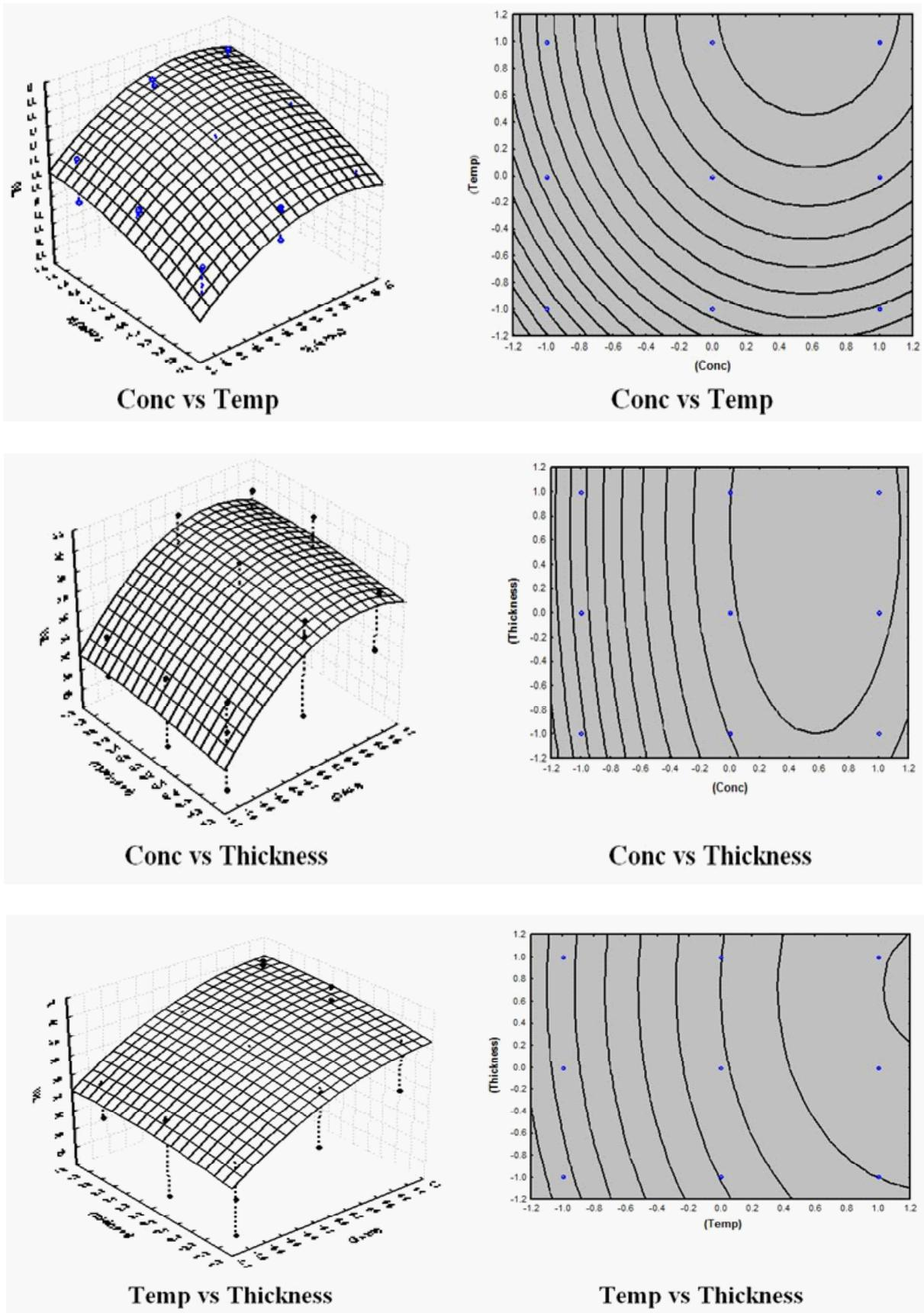
Figure 2. Response surface and contour plots showing the effect of processing variables on WL
