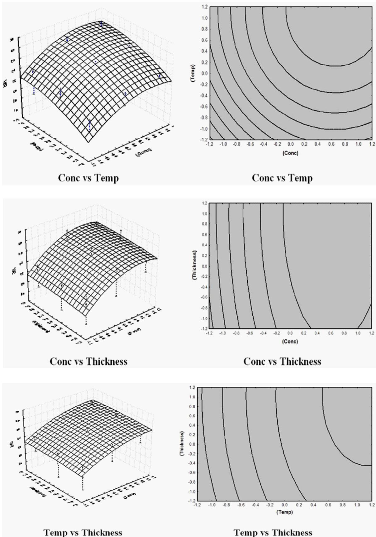
**Figure 6.** Response surface and contour plots showing the effect of processing variables on water reduction
