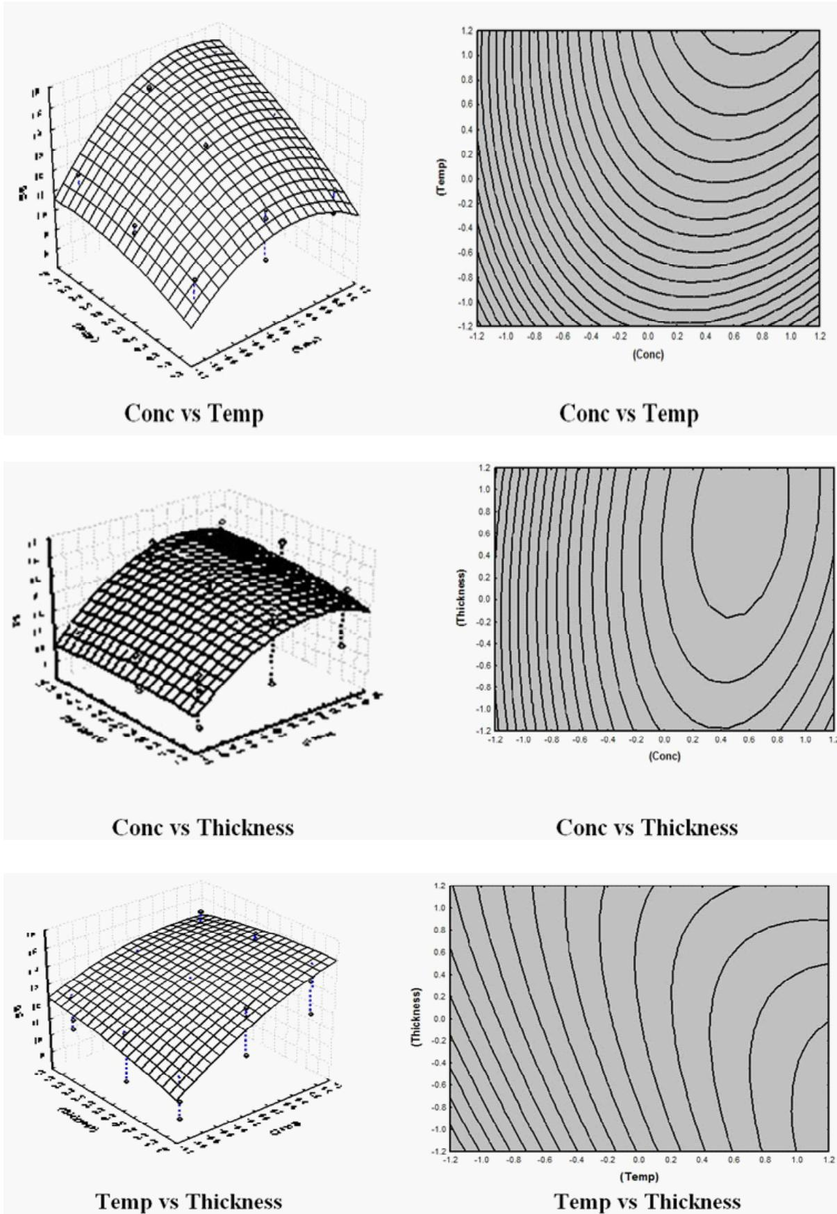
Figure 4. Response surface and contour plots showing the effect of processing variables on SG
