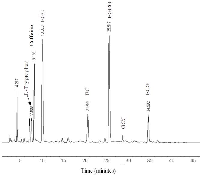
**Figure 3.** A representative HPLC chromatogram of a green tea sample run on a Shimadzu HPLC system with UV detection at 210 nm.
