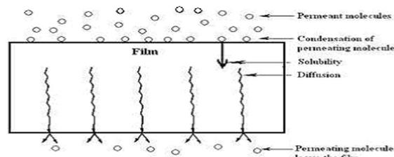
**Figure 7.** Scheme showing permeation of water vapor through a film
