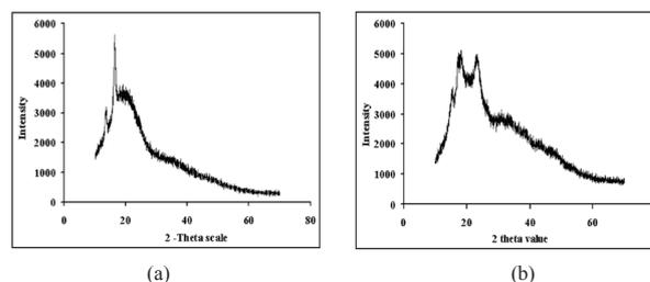
Figure 2(a). X-ray diffraction pattern for (a) Plain Sago starch film and (b) Sago starch powder
