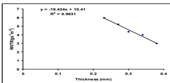
Figure 11. Plot between WVTR and thicknesses of films
