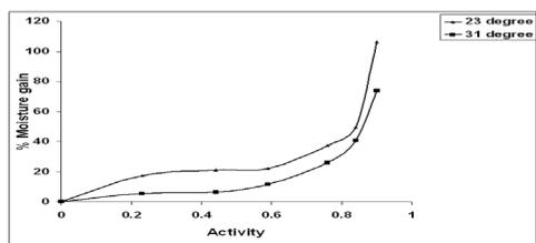
**Figure 4.** GAB Isotherm for plain sago starch film at different temperatures
