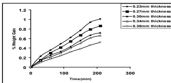
Figure 10. Effect of thickness on permeation of water vapor through films
