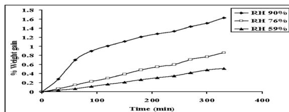
**Figure 5.** Kinetics of Water vapor permeation through PSS film at different RH and same temperature (28°C)
