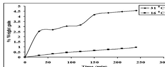
**Figure 6.** Kinetics of Water vapor permeation through PSS film at different temperature and same RH (100%)
