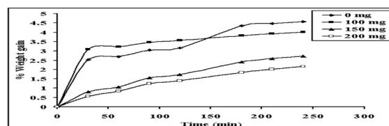
**Figure 8.** Effect of chitosan content on permeability of water vapor through film under relative humidity of 100 %, at 28°C
