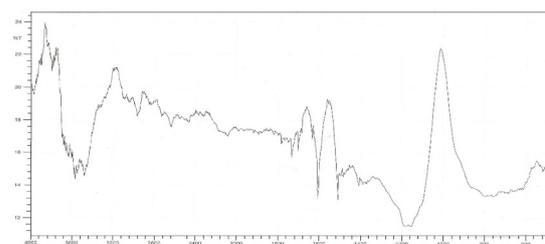
Figure 1. FTIR spectrum of glycerol plasticized sago starch film
