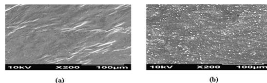
**Figure 9.** SEM images for (a) Plain sago starch film (b) Chitosan microparticles loaded sago starch film
