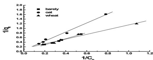
**Figure 1.** Langmuir isotherm plots for adsorption of MB by unsoaked straws (temperature = 30°C, contact time =180 min)
