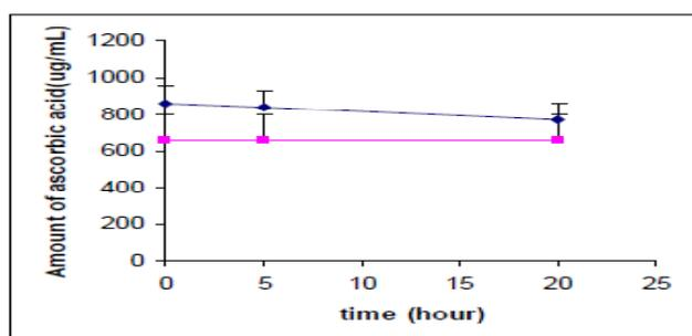
**Figure 2.** Correlation curve between amount of ascorbic acid and time (hr) of Kakadu plum.  $\diamond$ - $\diamond$  correlation curve of dried Kakadu plum ( $R^2 = 0.999$ )  $\circ$ - $\circ$  correlation curve of dried Kakadu plum plus 500  $\mu\text{g/mL}$  sodium metabisulphite
