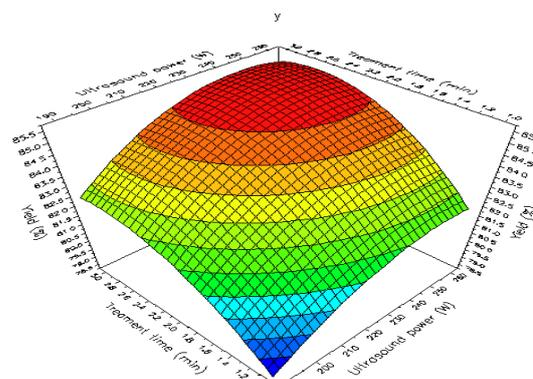
**Figure 4.** Response surface plot showing the effect of ultrasound power (W) and treatment time (min) on the extraction yield (%) in the pineapple juice processing with ultrasound-assisted extraction
