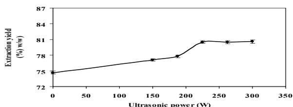
**Figure 1.** Effect of ultrasonic power on extraction yield in pineapple mash treatment
