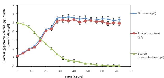
Figure 2. Time course of microbial biomass protein production and starch hydrolysis by *Candida utilis* NOY 1. All the experiments were carried out at 30°C, pH 5 and 150 rpm with 5g/L of starch. Fermentation was led 72 hours. Error bars show standard deviation among three observations. Values are means of triplicates  $\pm$  S.D. (Standard Deviation). The protein content is given in g of protein per 10 g of dried biomass.
