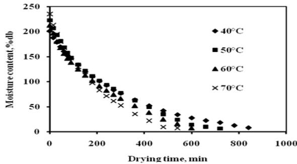
Figure 1. Variation of moisture content (dry basis) with drying time of stone apple slices dried by convective drying at different temperatures
