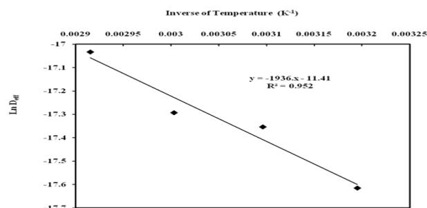
Figure 6. Plotting of effective moisture diffusivity for estimation of activation energy
