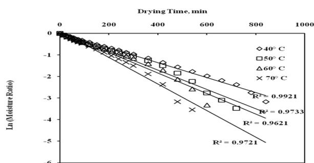
Figure 5. Linear relationship between  $\ln(MR)$  and drying time at various drying temperatures
