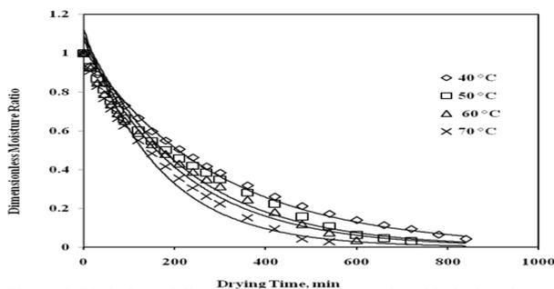
Figure 3. Variation of dimensionless moisture ratio with drying time of stone apple slices dried at different temperatures
