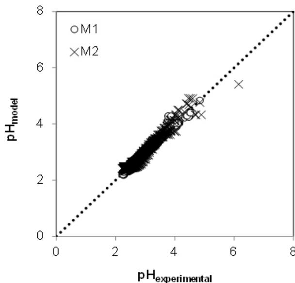
Figure 2. Evaluation of the proposed models using Equation 3. M1 is Equation 1 and M2 is Equation 2. The dots are the obtained data (model versus experimental) and the dashed line represents a regression with  $\alpha = 1$ ,  $\beta = 0$  and  $R^2 = 1$
