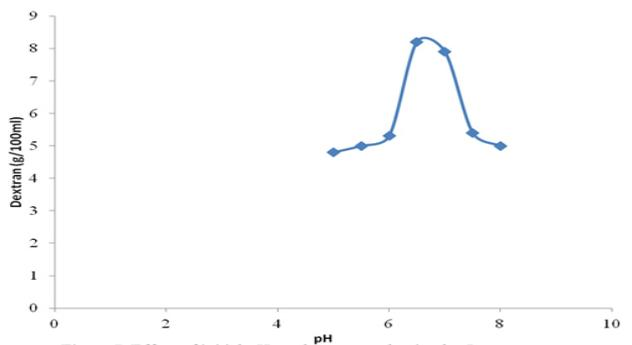
Figure 7. Effect of initial pH on dextran production by *Leuconostoc* spp.
