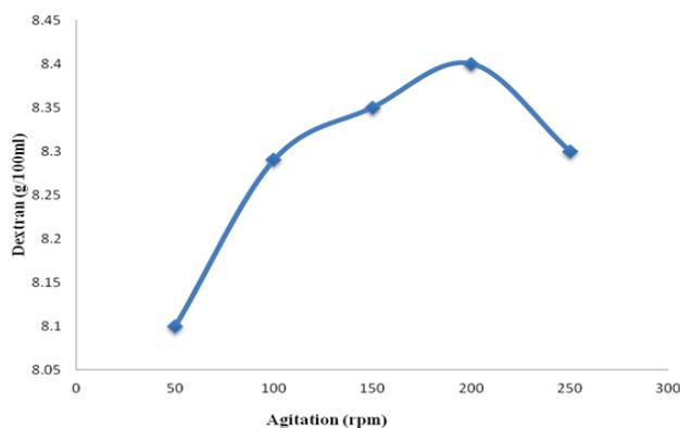
Figure 8. Effect of agitation speed on dextran production by *Leuconostoc* spp.
