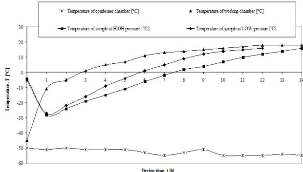
Figure 3. Change of temperature at freeze-drying of lemon balm leaves (shift the horizontal axis)
