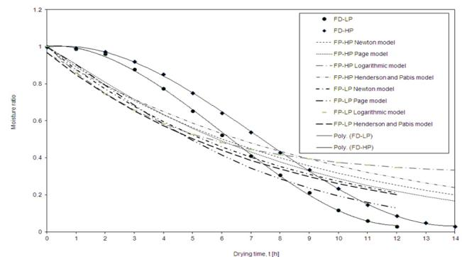
Figure 2. Variations of moisture ratio as a function of time for freeze drying of lemon balm
