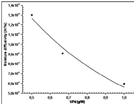
Figure 5. Variation of effective diffusivity as function of power densities
