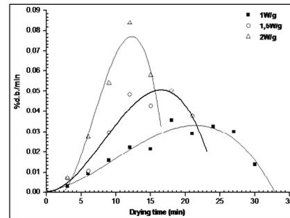
Figure 2. Variations of drying rate at different microwave power densities
