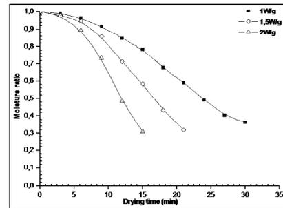
Figure 1. Drying curves of moisture ratio with drying time at different microwave power densities
