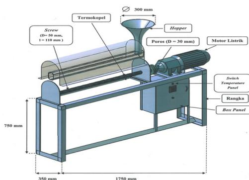
Figure 1. Single screw conveyer
