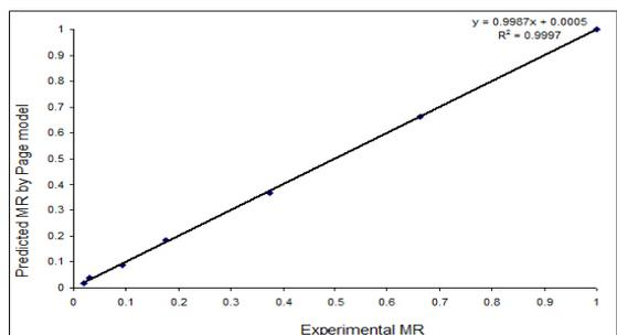
Figure 4. Predicted MR versus Experimental MR by Page model at 80°C
