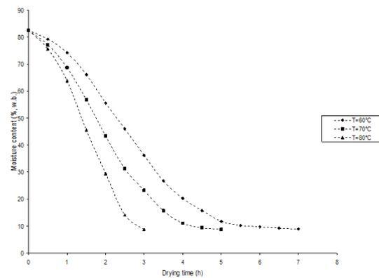
Figure 1. Effect of drying temperature on the moisture content of mango slice
