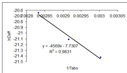
Figure 6. Arrhenius-type relationship between effective diffusivity and temperature.
