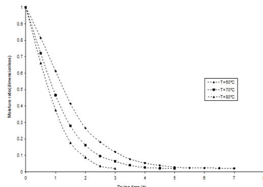
Figure 2. Effect of drying temperature on the moisture ratio of mango slices.
