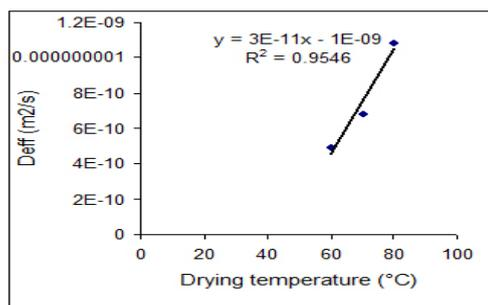
Figure 5. Effect of drying temperature on the effective diffusivity of water in mango slices
