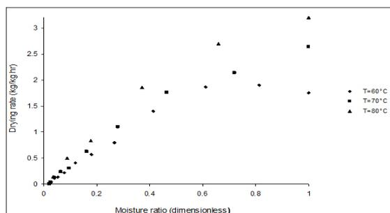
Figure 3. Drying rates versus the experimental moisture ratio of mango slices
