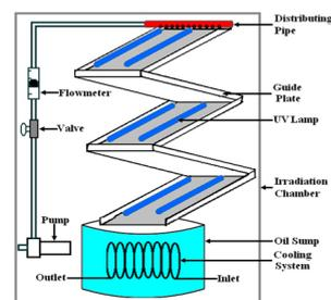
Figure 1. Diagram of experimental photo-degradation reactor
