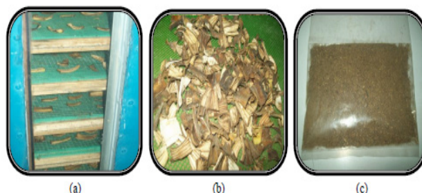
Figure 2. Saba banana peel powder preparation. (a) oven-drying of banana peels (b) banana peels after drying (c) banana peels after grinding
