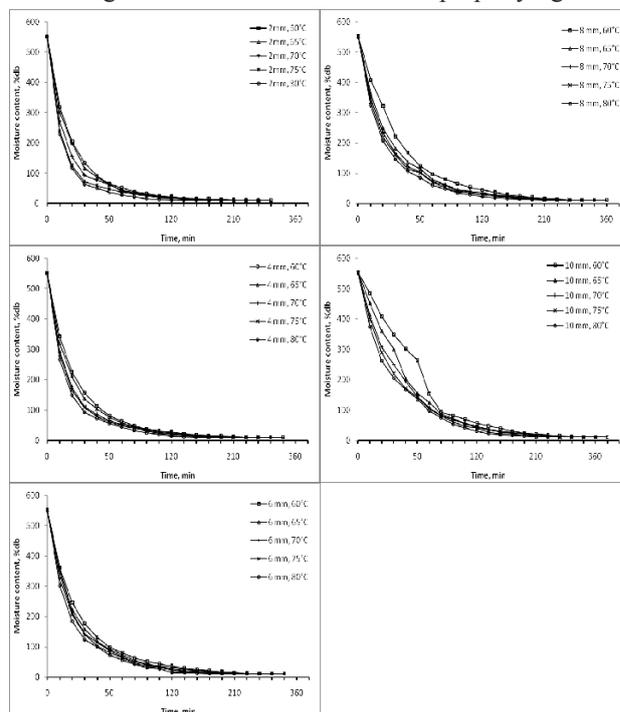
Figure 2. Thin layer drying curves of bael fruit pulp at various thickness and temperatures
