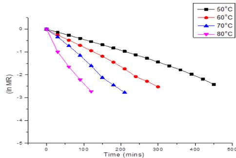
Figure 2. A plot of ln MR and time of jackfruit at different temperatures
