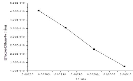
Figure 3. Variation of effective diffusivity with absolute temperature
