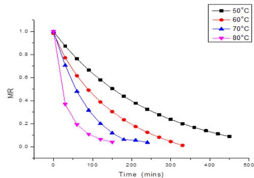
Figure 1. A plot of moisture ratio and time for experimental data of jackfruit at different temperatures
