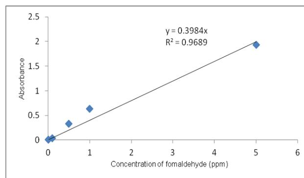
Figure 1. Calibration curve of standard formaldehyde solution
