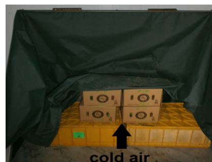
Figure 1. Forced-air cooling setup for precooling the Berangan banana. A mounted fan that located at the back forced the cold air passed through the packages and bananas and out through the fan. Two parallel rows of banana were covered by a plastic strip so that it can force as much cold air pass through the actual product as possible
