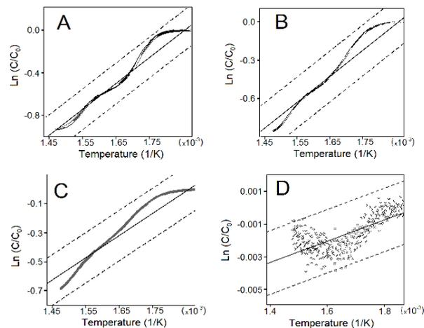
Figure 3. Regression equation of gallic acid decomposition at 10 °C/min (A), 15 °C/min (B), 20 °C/min (C), and 25 °C/min (D)
