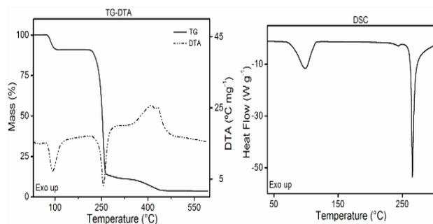
Figure 1. Simultaneous TG-DTA curves (left) and DSC curve (right) of gallic acid
