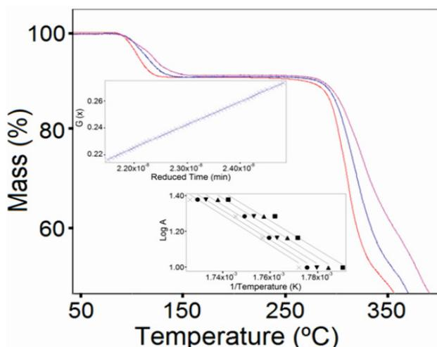
Figure 2. TG curves on kinetic values in the thermal decomposition of gallic acid at heating rates of 10, 15, 20 and 25 °C min<sup>-1</sup>
