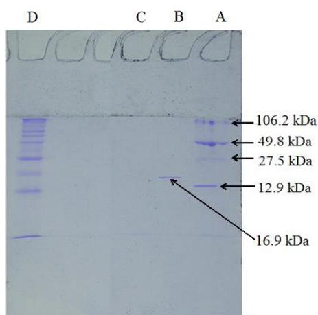
Figure 4. SDS-PAGE analysis: in lane A bands achieved after purification with acetone, in lane B, after purification with phenyl-sepharose gel, in lane C after purification with sephadex G-100, and lane D represents SDS-PAGE results for the standard molecular weight markers
