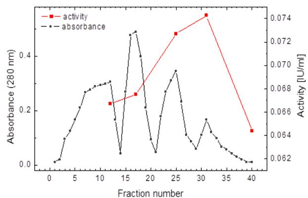
Figure 3. Purification of cellulase using Sephadex G-100 column 0.01 M Tris-HCl buffer, pH 8.0 at a flow rate of 24 ml/h. Column size was (2.5×1.8 cm)
