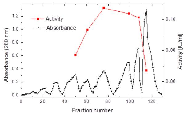
Figure 2. Absorbance at  $\lambda = 280$  nm of the fractions showing enzyme activity (left); calculated enzyme activity for the tubes with the highest optical densities (right). Enzyme solution was added to the phenyl-sepharose gel. Column size was (2.5×1.8 cm), the flow rate was 15 ml/h, 0.01 M Tris-HCl buffer, pH 8.0 containing a gradient of 1, 0.6, 0.4 0.2 M of ammonium sulphate
