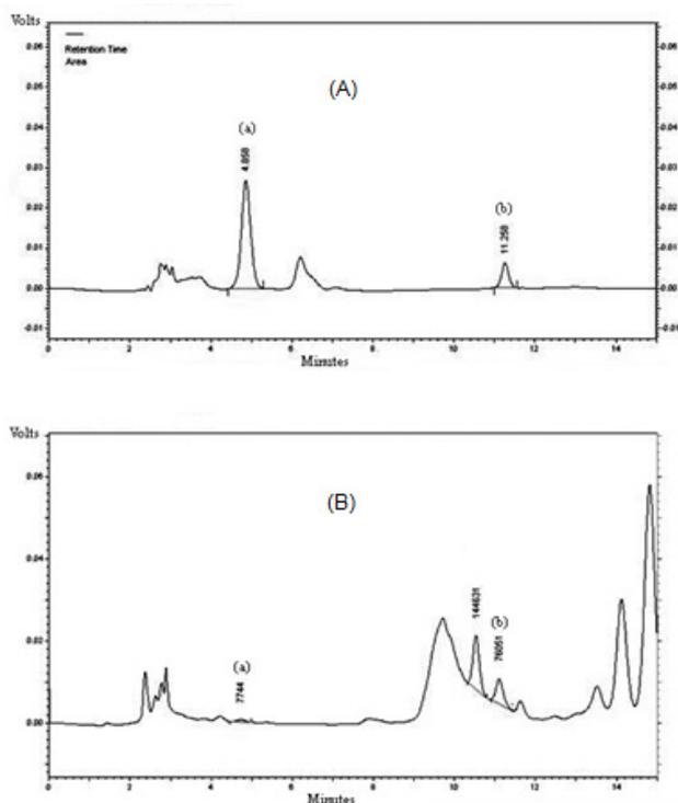
Figure 1. (A) chromatogram of a standard mixture of retinol (a) and alpha tocopherol (b), each at a concentration of  $10 \text{ mg L}^{-1}$ ; (B) chromatogram of corn oil nanoemulsion sample
