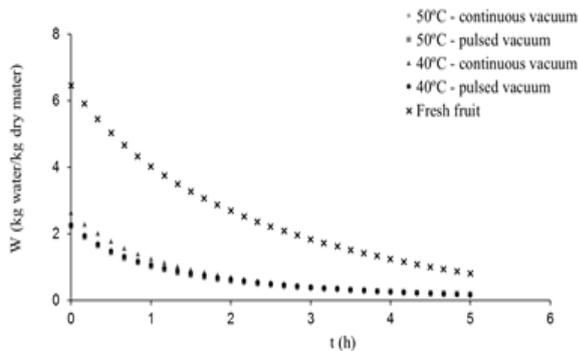
Figure 2. Effect of osmotic pretreatment on guava moisture content (d.b.) during convective drying
