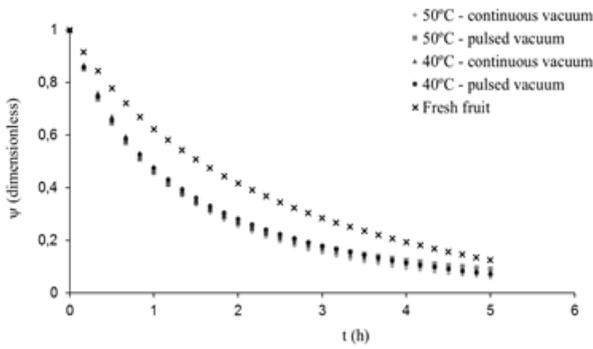
Figure 1. Effect of osmotic pretreatment on guava dimensionless moisture content during convective drying
