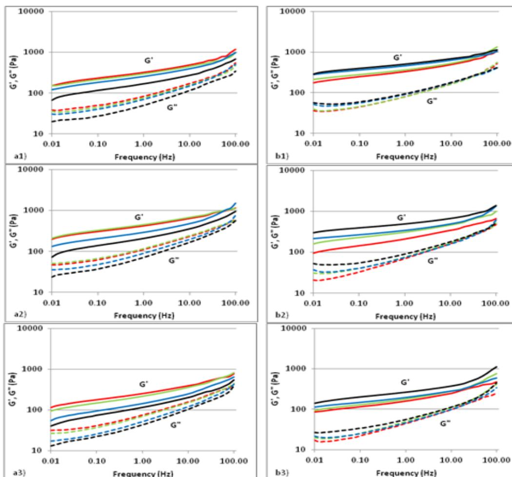
Figure 3. Storage modulus ( $G'$ , solid line) and loss modulus ( $G''$ , dashed line) of frequency sweep test of puddings from different formulations: GF-HPJF (a1); SF-HPJF (a2); CF-HPJF (a3); GF-LPJF (b1); SF-LPJF (b2); and CF-LPJF (b3) on day 0 (—), 2 (—), 8 (—) and 16 (—).  $n = 3$ .
