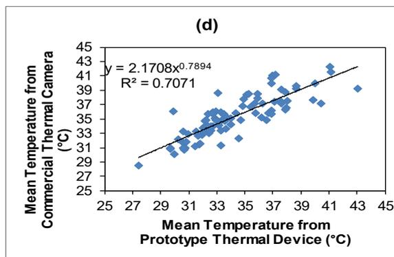
Figure 4. Scatter plot of mean temperature from commercial thermal camera versus mean temperature from prototype thermal device of (a) Under-ripe FFB, (b) Ripe FFB, (c) Over-ripe FFB and (d) All FFB
