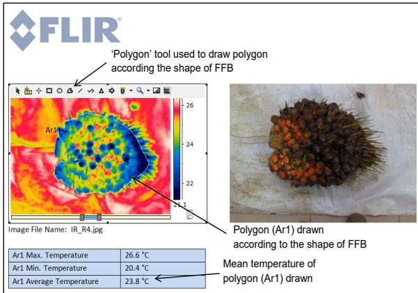
Figure 1. Mean temperature of FFB thermal image determined by polygon drawn in the report created by ‘FLIR Reporter’ with the thermal image on left and the corresponding digital image on right
