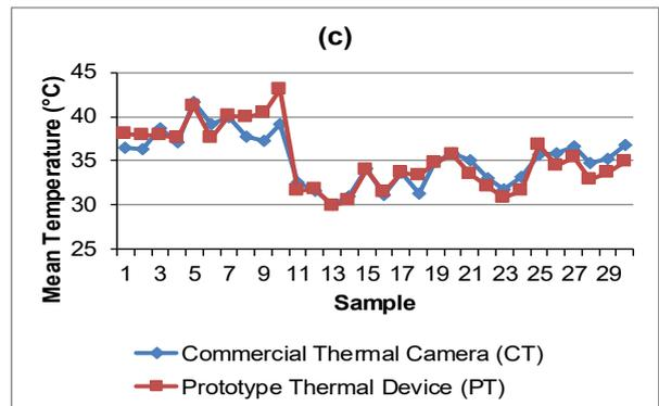
Figure 2. Line chart of mean temperature from prototype thermal device and commercial thermal camera for (a) Under-ripe FFB, (b) Ripe FFB and (c) Over-ripe FFB
