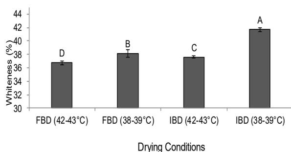
Figure 6. Whiteness degree (%) from FBD and IBD at 38-39°C and 42-43°C. [Means followed by the different letters within a column are significantly different ( $P < 0.05$ )].
