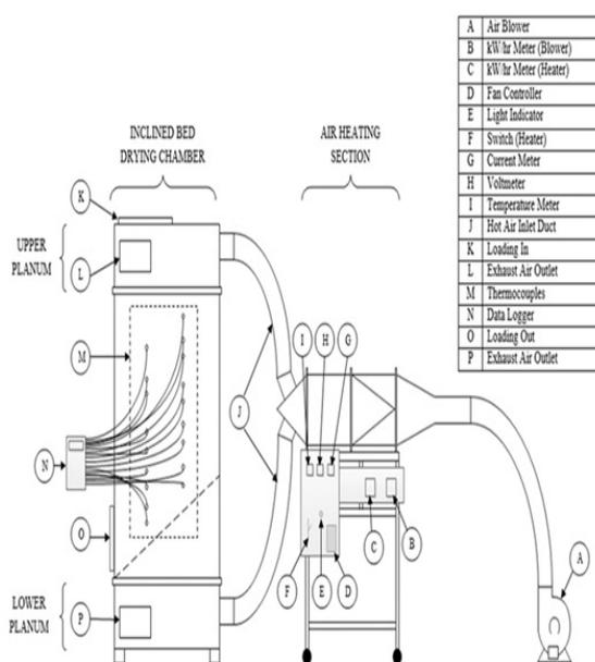
Figure 1. Schematic diagram of drying system.
