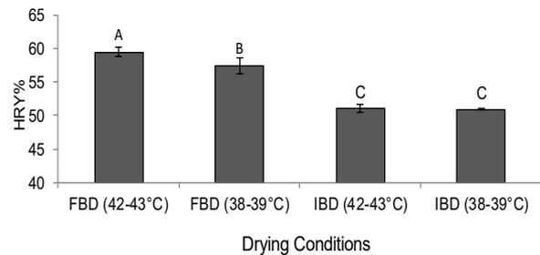
Figure 5. Head rice yield (%) from FBD and IBD at 38-39°C and 42-43°C. [Means followed by the different letters within a column are significantly different ( $P < 0.05$ )].
