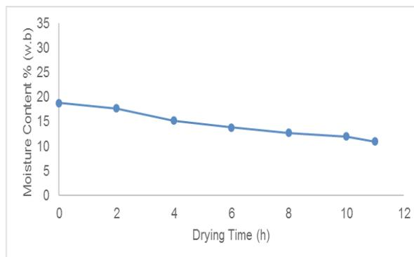
Figure 2b. Drying Curve of FBD at 42-43°C .
