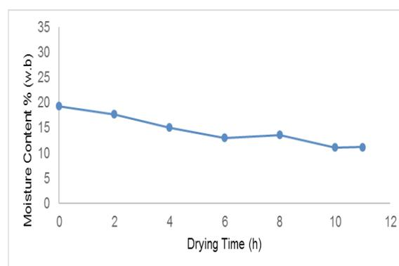
Figure 3b. Drying Curve of IBD at 42-43°C.
