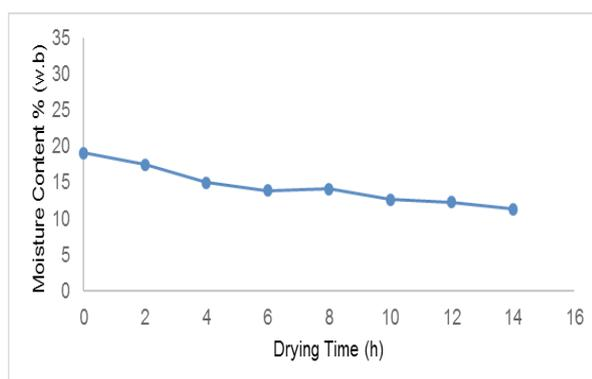
Figure 3a. Drying Curve of IBD at 38-39°C.
