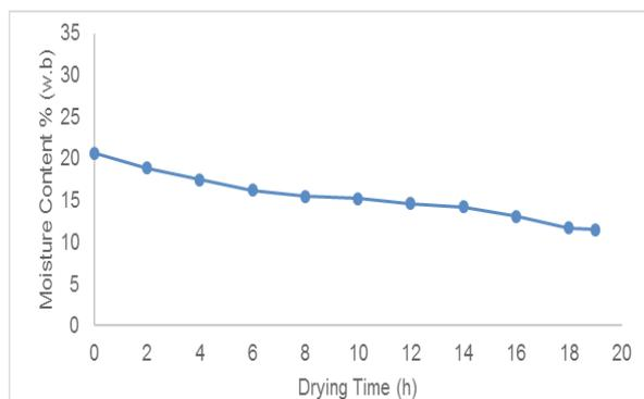
Figure 2a. Drying Curve of FBD at 38-39°C .
