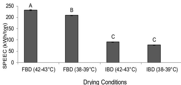
Figure 4. Specific electrical energy consumption of FBD and IBD at 38-39°C and 42-43°C. [Means followed by the different letters within a column are significantly different ( $P < 0.05$ )].
