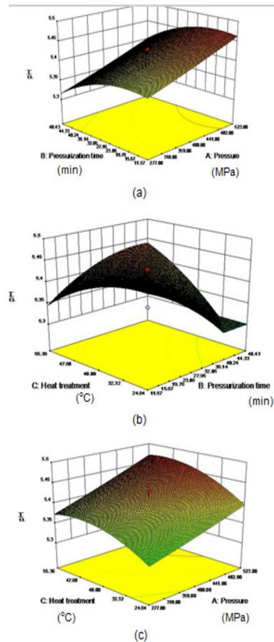
Figure 2. Response surface plots showing effect on pH of the acidified milk gels: (a) pressure and pressurization time, (b) pressurization time and heat treatment, and (c) pressure and heat treatment
