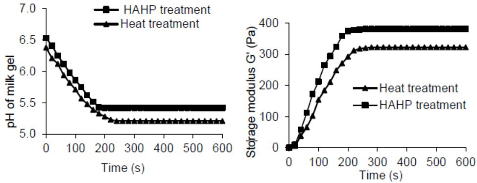
Figure 1 Variation in pH and storage modulus of the acidified milk gel with time at 400 MPa for 30 min at 40°C
