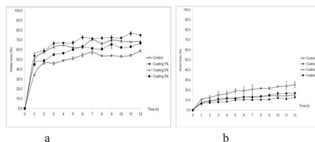
Figure 2. Water Loss (a) and Solid Gain (b) of non-coated pumpkin and coated pumpkin with 1%, 2% and 3% sodium alginate during osmotic dehydration
