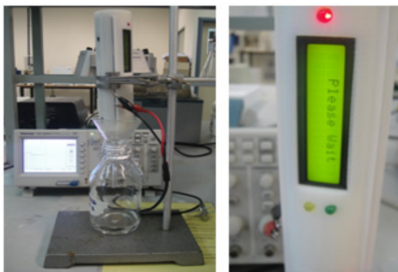
Figure 2. The portable E-Nose prototype (Length=21cm, width=7 cm, thickness= 5 cm)
