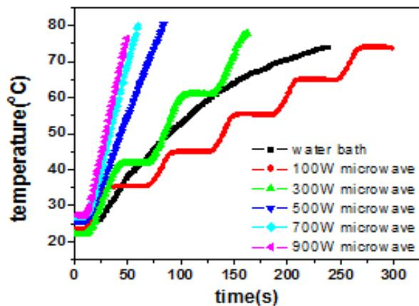
Figure 3. Temperature-time curve for WBH (black) and MH (at 100 W, 300 W, 500 W, 700 W and 900 W microwave power) of 500 ml distilled water
