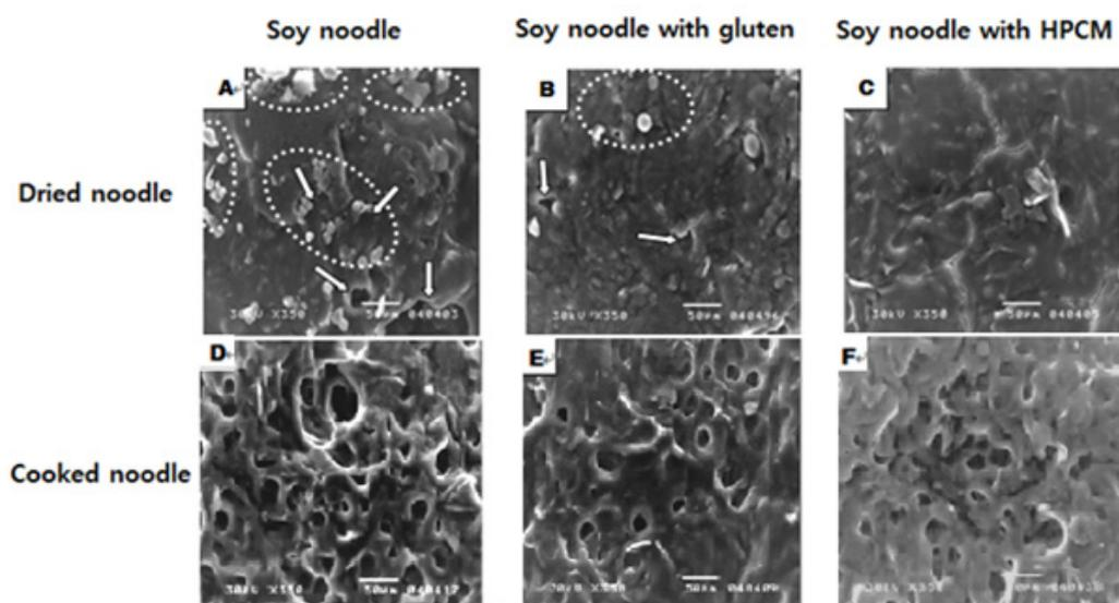
Figure 2. The scanning electron micrographs of the surface of the dried noodles (A-C) and the cross-section of the cooked noodles (D-F). A: Dried soy noodle, B: Dried soy noodle with gluten, C: Dried soy noodle with 1.5% HPMC, D: Cooked soy noodle, E: Cooked soy noodle with gluten, F: Cooked soy noodle with 1.5% HPMC.
