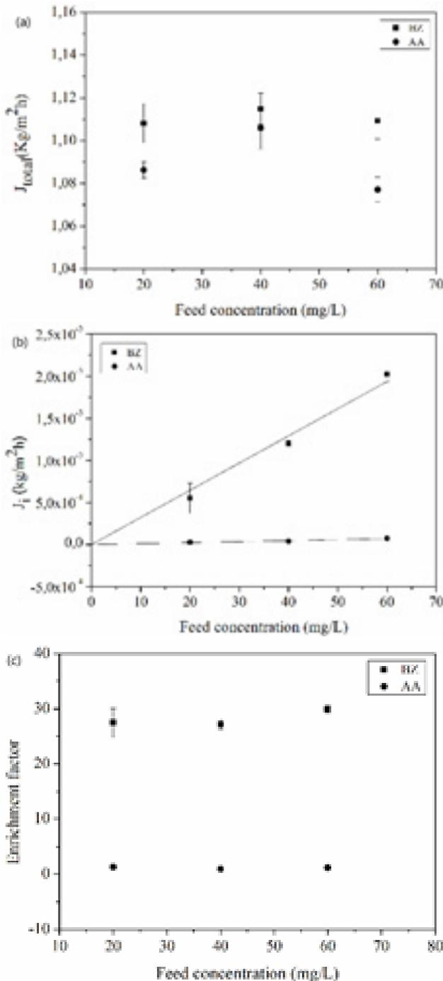
Figure 3. Feed concentration effect on (A) total flux, (B) individual permeation fluxes for benzaldehyde and acetic acid, and (C) benzaldehyde and acetic acid enrichment factor.
