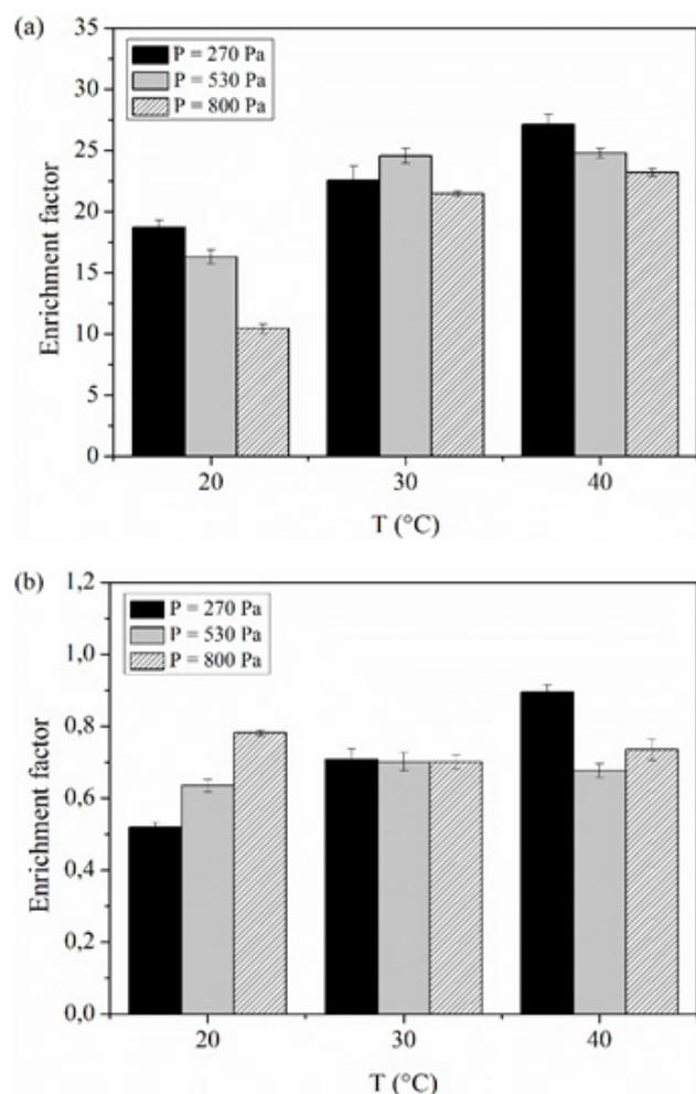
Figure 2. Feed temperature effect on binary solutions enrichment factor at different permeate pressures (feed flux rate = 3.0 L/min) for benzaldehyde (A), and acetic acid (B).
