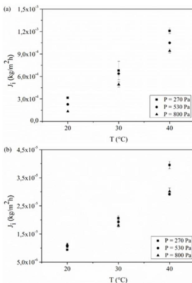
Figure 1. Feed temperature effect on individual permeation fluxes for benzaldehyde (A), and acetic acid (B).
