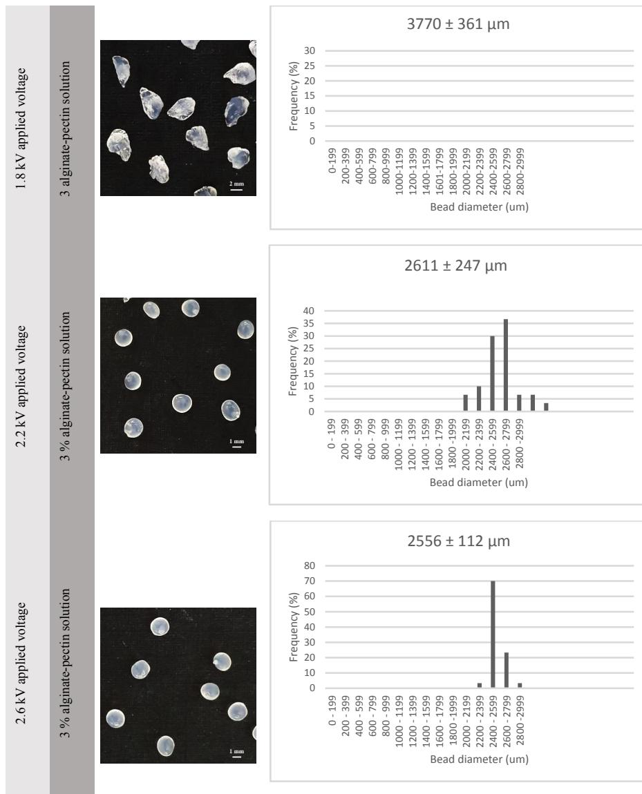
Figure 1. Optical images and size distributions of alginate-pectin beads of selected samples at three different applied voltages (1.8, 2.2, and 2.6 kV).
