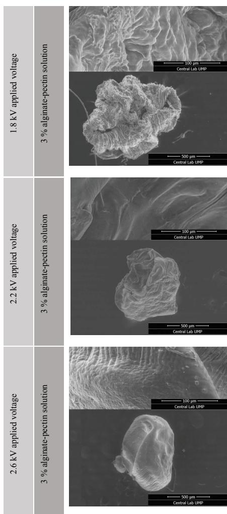
Figure 2. SEM photographs of alginate-pectin beads of selected samples at three different applied voltages (1.8, 2.2, and 2.6 kV).
