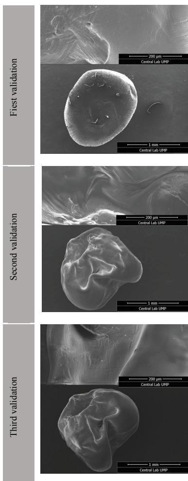
Figure 4. SEM photographs of alginate-pectin beads as validation experiments at desirability values of 0.711, 0.701, and 0.677, respectively.
