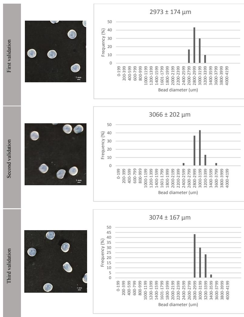
Figure 3. Optical images and size distributions of alginate-pectin beads as validation experiments at desirability values of 0.711, 0.701, and 0.677, respectively.
