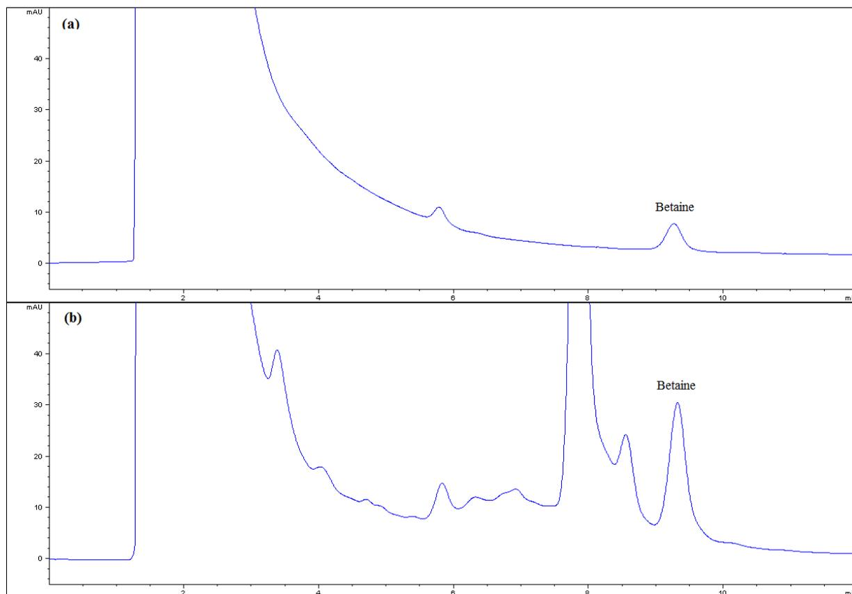
Figure 2. HPLC chromatograms of (a) standard solution of betaine hydrochloride (5.86 mg/L), and (b) betaine (23.90 mg/L) in goat milk sample.
