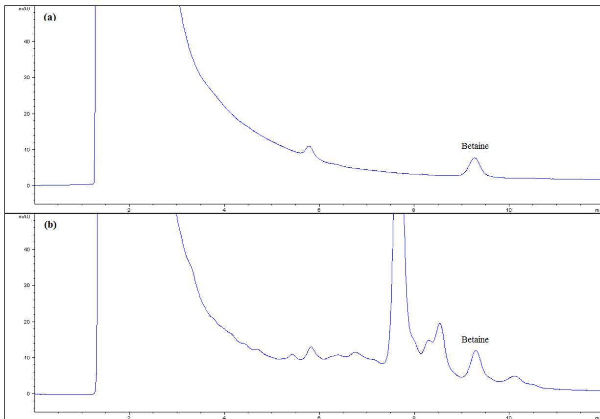
Figure 1. HPLC chromatograms of (a) standard solution of betaine hydrochloride (5.86 mg/L), and (b) betaine (7.85 mg/L) in cow milk sample.
