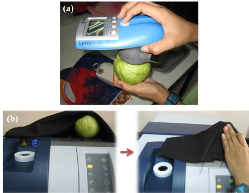
Figure 2. The measurement of (a) the optical reflectance, and (b) near infrared absorbance showing the placement of the guava sample covered with black cloth to prevent surrounding light from entering the scanning window.
